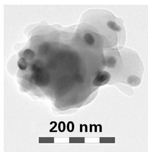
**Fig. 4:** TEM-image of a 350 nm furniture coating particle with firmly embedded nanoscaled ZnO additive particles, released during sanding.
