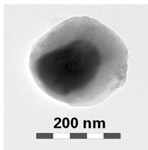
**Fig. 5:** TEM-image of a 200 nm sanding aerosol particle, where a single TiO<sub>2</sub> pigment particle is sheathed completely by the matrix material.
