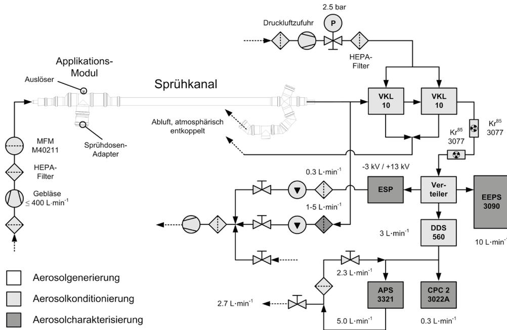
**Fig. 3:** Schematic illustration<sup>9</sup> of the experimental setup used for the release characterisation during spray application of liquid coatings (APS = time-of-flight spectrometer, CPC = condensation nuclei counter, EEPS = fast measuring electrical mobility spectrometer, VKL/DDS ... dilution units, ESP ... electrostatic precipitator for subsequent electron microscopy).
