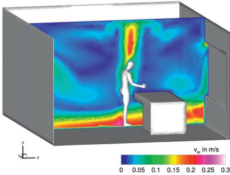
**Fig. 7:** Visualisation of the mean steady-state flow velocity through the working area in case of natural ventilation by opened pivot-hung window (air exchange rate 1.5 h<sup>-1</sup>, temperature specifications: 5°C inlet air, 20°C mean room temperature via floor heating, 26°C clothing surface, 30°C hand surfaces, 35°C head surface).
