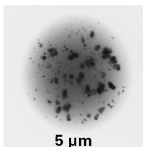
**Fig. 6:** TEM-image of a dried acrylate spray droplet from a propellant spray can with embedded nanoscaled ZnO additive particles and non-nanoscaled TiO<sub>2</sub> pigment particles.
