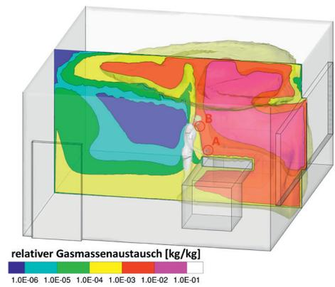
**Fig. 8:** Calculated aerosol propagation 75 s after spray application of a liquid coating by a propellant spray can within a 5 m x 6 m x 3 m = 90 m<sup>3</sup> model room ventilated by an opened pivot-hung window (air exchange rate 1.5 h<sup>-1</sup>) and closed door; A = region of release, B = region of exposure (breathing zone).
